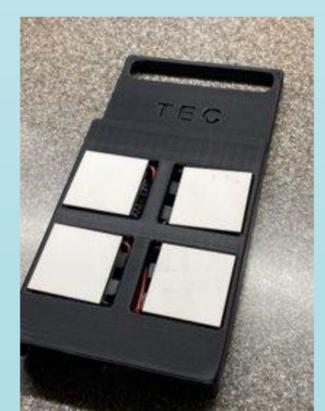
Figure 6. Case with four Peltier tiles
