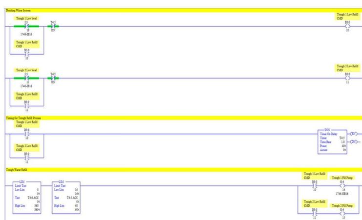
Figure 3. PLC Ladder Logic on SLC500
